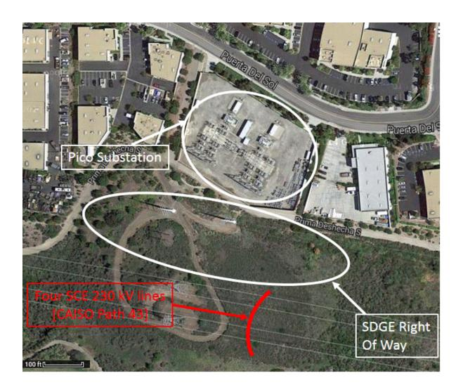
FIGURE 5: ALTERNATIVE 2 CONFIGURATION FOR CONNECTING 230 KV LINES TO SDGE'S PICO SUBSTATION WITH FOUR 138 KV CONNECTIONS TO PICO.
